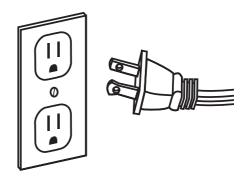
**A WARNING:** It is normal for the power cord to feel warm to the touch. However, a loose fit between the outlet and the plug may cause overheating of the plug. If this occurs, try inserting the plug into a different outlet. Contact a qualified electrician to inspect the original outlet for damage.
