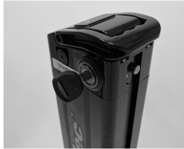
Key at position B Battery locked
