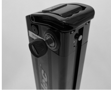
Key at position B Battery locked
