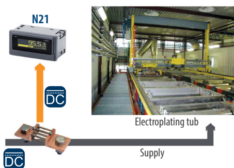
Current measurement in an electroplating plant
