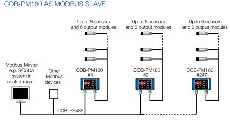
Each COB-PM180 is a slave device on the main network and the master on each network of sensors.
