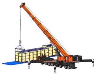
Vertical portrait package unloading with crane
