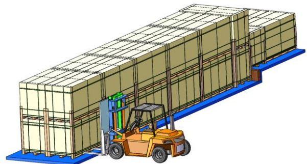
Vertical landscape package unloading with forklift
