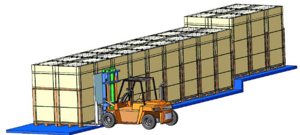
Vertical portrait package unloading with forklift
