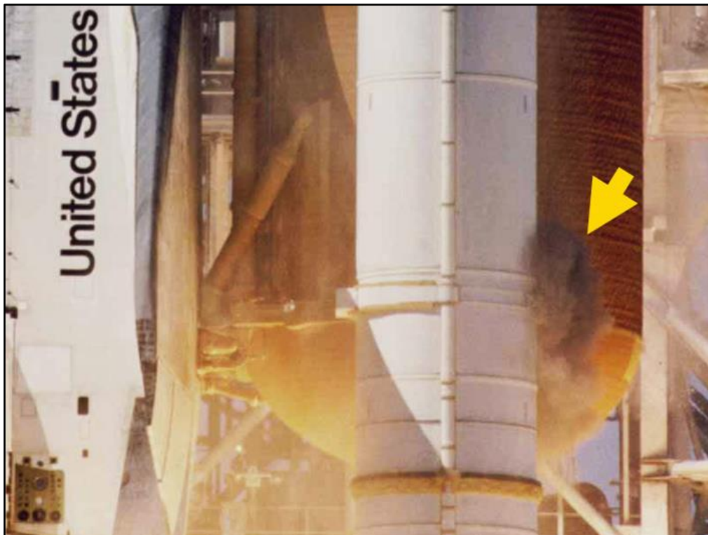
Figure 2.8 The Space Shuttle Challenger exploded soon after launch when a faulty seal in the solid rocket booster caused a catastrophic failure. The contractor/manufacturer of the part had advised NASA that due to the cold weather being experienced at the time of launch, it could not guarantee the integrity of the part and recommended a delay until the weather became warmer. Upon pressure from NASA, the management at the contractor decided that perhaps the risk was acceptable and gave the go-ahead even though later they would admit that the recommendation was probably not appropriate. The image above shows black smoke emanating from the faulty seal during the launch sequence.
