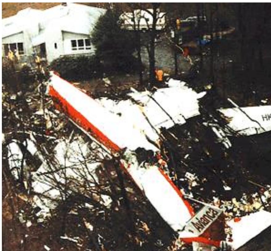
Figure 2.13. Avianca Flight 52, a Boeing 707, crashed on Long Island near New York whilst attempting an approach to JFK. The crew did not assert themselves within their team environment and to ATC when it was apparent that they did not have the fuel to make a go around and return for landing under ATC instructions. (Photo origin unkn)
