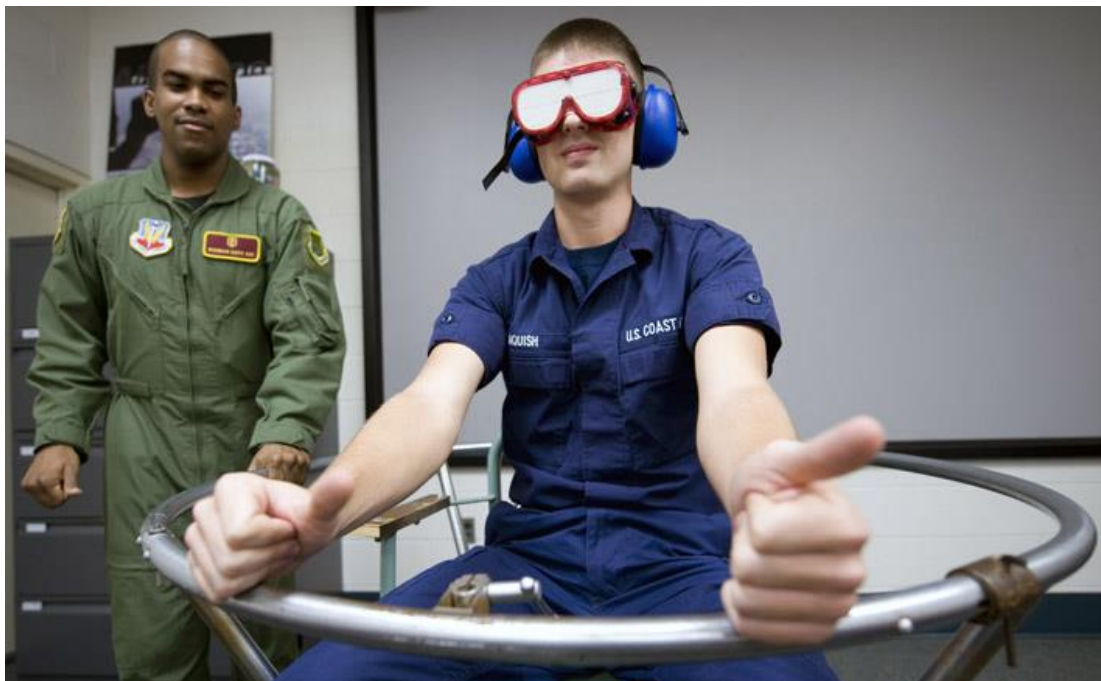
Figure 3.46 115 A Barany Chair is used to demonstrate spatial disorientation to US Air Force cadets.
