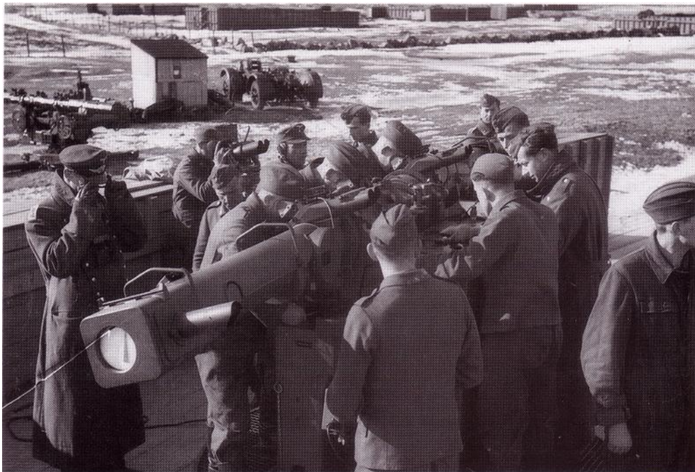
Figure 3.32 85 German Anti-Aircraft range and altitude finder. The wider the distance between the individual optics, the more accurate is the range finding ability. Here, German Grenadiers look through the rangefinder. Once enemy aircraft are spotted, the optics are focussed so that the image is clear and are not double vision. This requires movement of the lens and movement of the angle of the mirrors. It is this angular movement that gives the single vision and provides the trigonometric information to determine how far the object being viewed is. With this information, the angle from the horizontal is attained which can then give the altitude using trigonometry again. The placement of the eyes on the human face is a smaller version of this.
