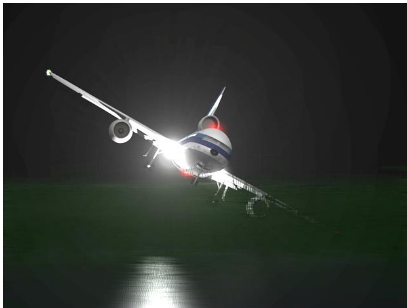
Figure 4.10 Eastern Airlines Flight 401 – its left wingtip about to impact the Everglades Swamp – was completely serviceable and airworthy except for a $12.00 light which was the factor that started the chain reaction that caused the accident.
