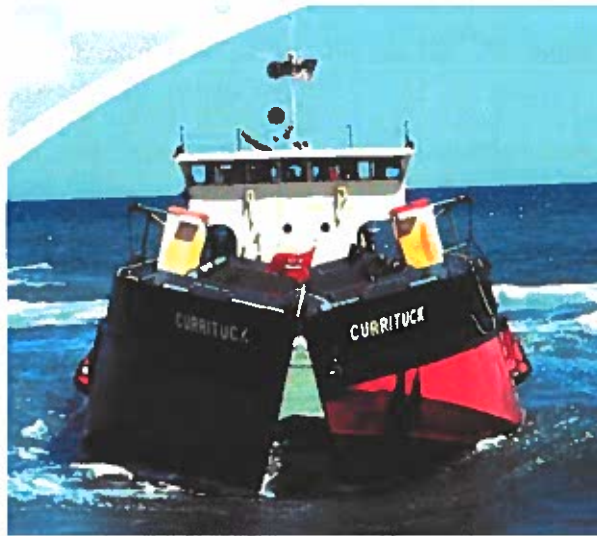
Figure 2-20. USACE Shallow Draft Split-Hull Hopper Dredge the Currituck Rarely Dredges the LWF Inlet
