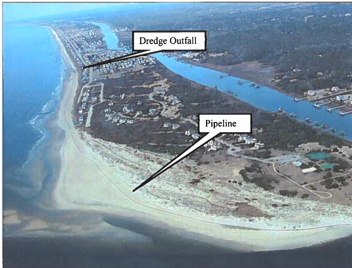
Figure 2-13. Aerial Photograph of 2014 LWFIX Nourishment [source: NC Division of Coastal Management (DCM)].
