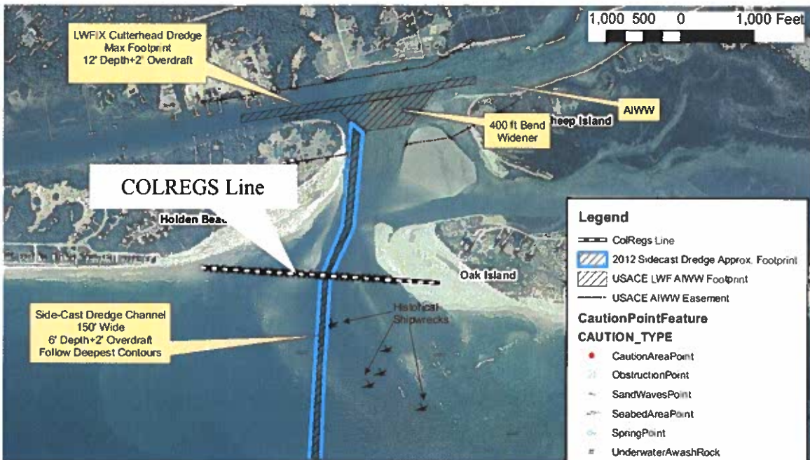
Figure 2-21a. LWF Inlet USACE Dredging Projects Include the Outer Channel (sidecaster dredged) and the LWFIX (cutterhead dredged)
