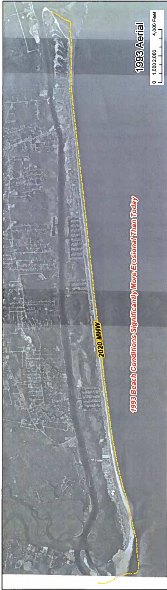
Figure 3-14 1993 and 2019 Aerial Comparison with 2020 Mean High Water (MHW) line. 2019 aerial and 2020 MHW Line shows overall accretion in comparison with 1993 conditions.
