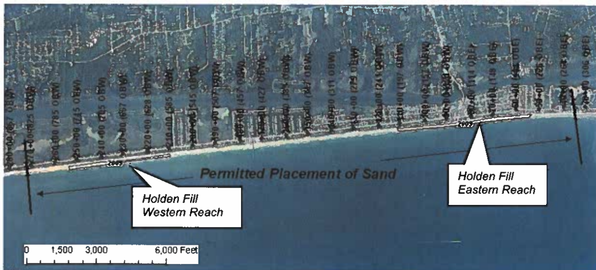
Figure 2-2. 2009 Constructed Project Reaches and 2009 Permitted Sand Placement (the permitted placement has been modified over the years)
