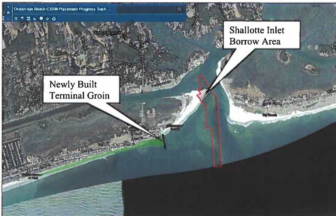
Figure 3-11. Ocean Isle Beach 2021/2022 Terminal Groin and Federal CSRM Beach Renourishment Projects. Shallotte Inlet Borrow Area and Placement Area Shown (USACE Ocean Isle Beach CSRM Placement Progress Tracker)
