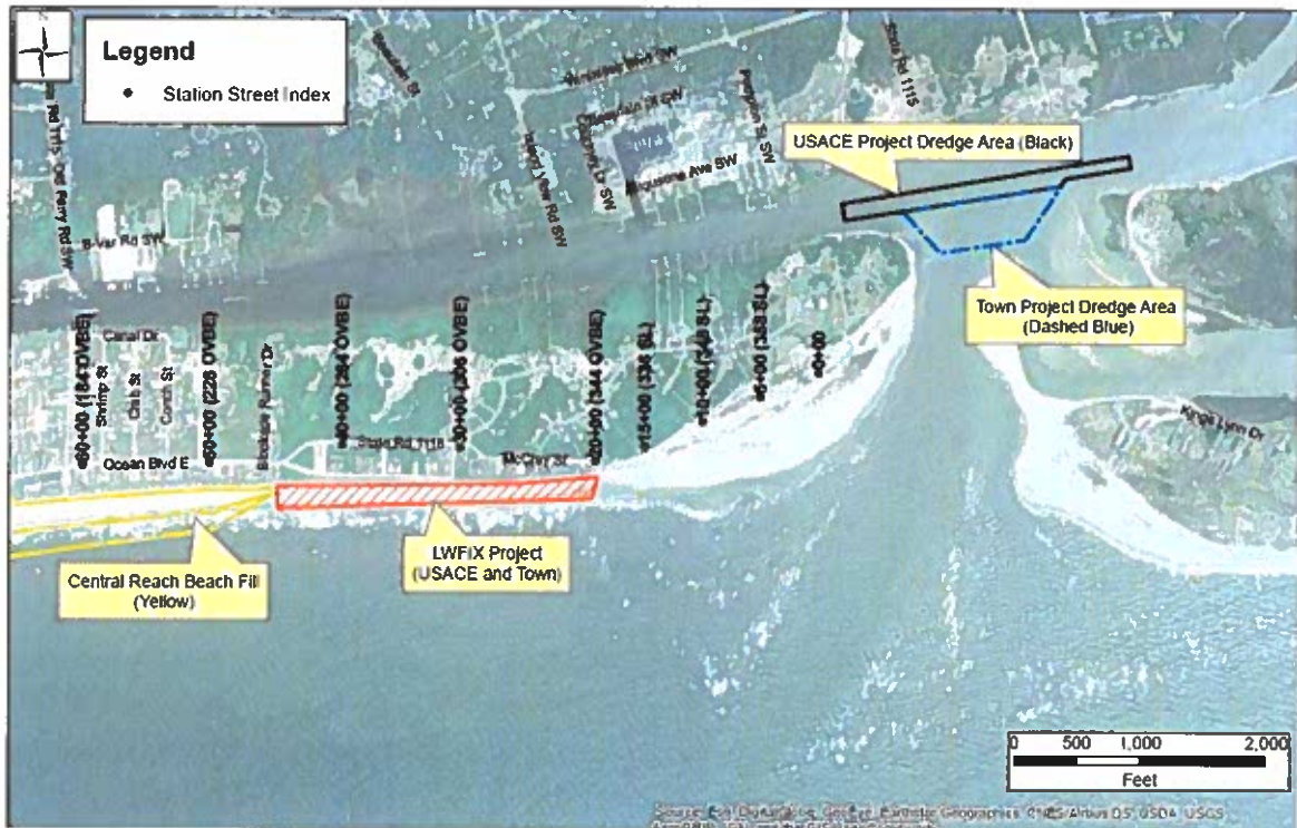
Figure 2-14. 2017 USACE LWFIX Dredging and Beach Placement Schematic (source USACE request for proposal). Placement of Approximately 120,000 cy occurred in March 2017 between Holden Beach Stations 20+00 and 45+00 to meet in with the Central Reach Project.
