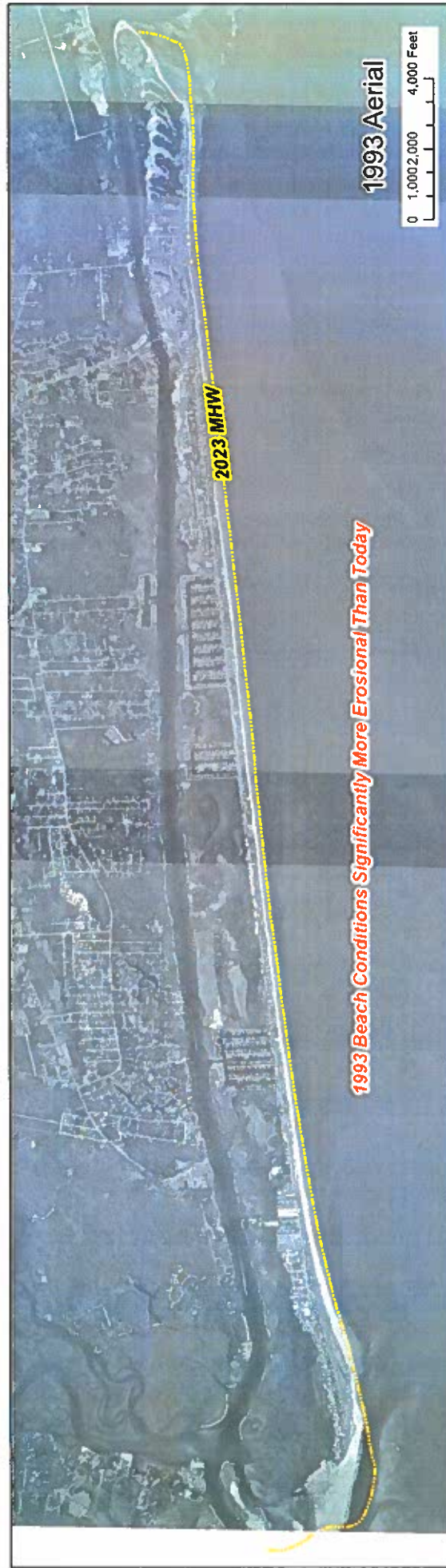
Figure 3-15 1993 and 2023 Aerial Comparison with 2023 Mean High Water (MHW) line. 2023 aerial and 2023 MHW Line shows overall accretion in comparison with 1993 conditions.
