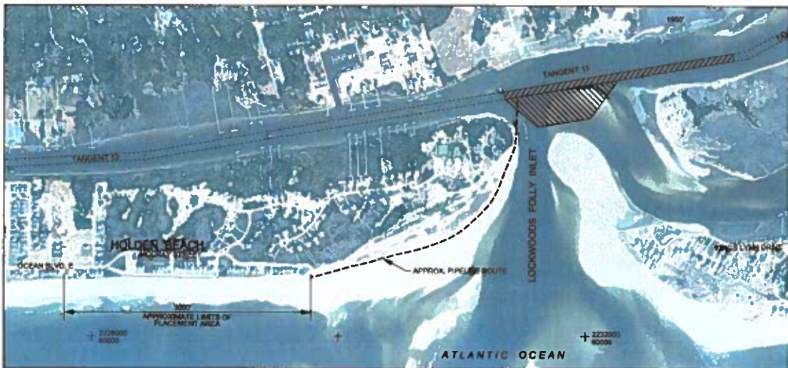
Figure 2-20. 2020 LWFIX Placement on Holden Beach. 400-ft Bend Widener Included as Bid Option Item (Alt) But Was Only Lightly Dredged During Actual Project.
