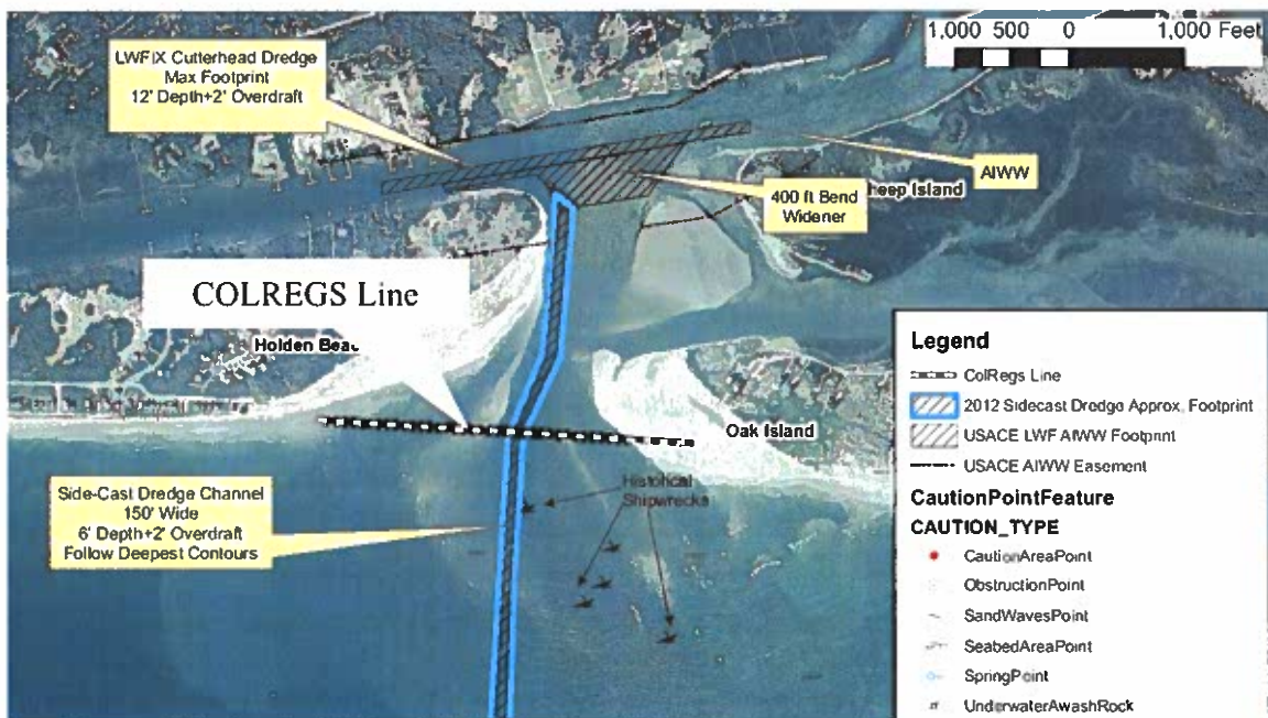
Figure 2-26 (A). LWF Inlet USACE Dredging Projects Include the Outer Channel (sidecaster dredged) and the LWFIX (cutterhead dredged)
