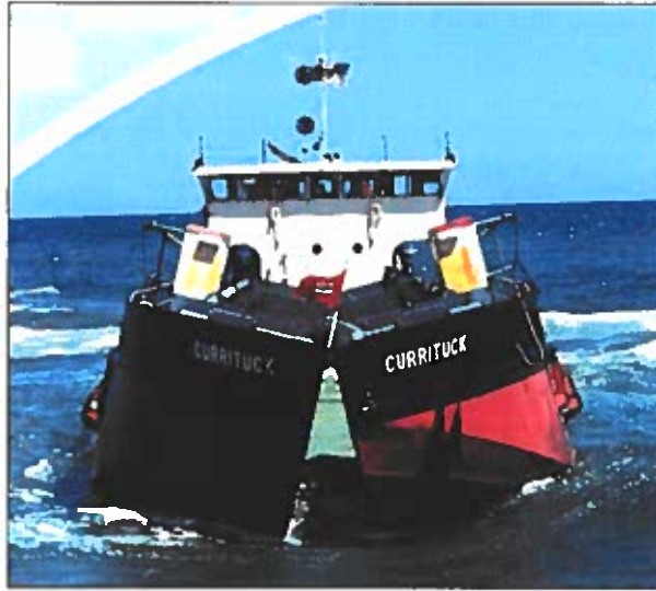
Figure 2-25. USACE Shallow Draft Split-Hull Hopper Dredge the Currituck Rarely Dredges the LWF Inlet
