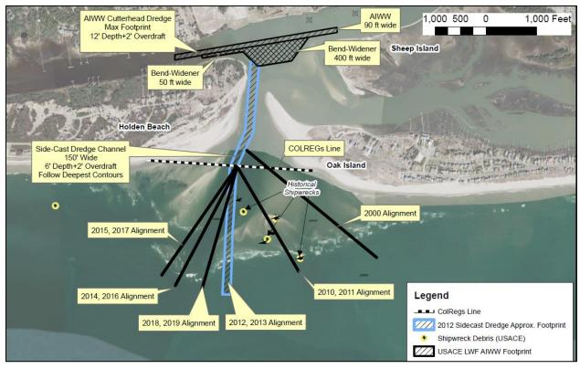
Figure 1-3. LWF Inlet Outer Ebb Channel Alignments and Bend-Widener
