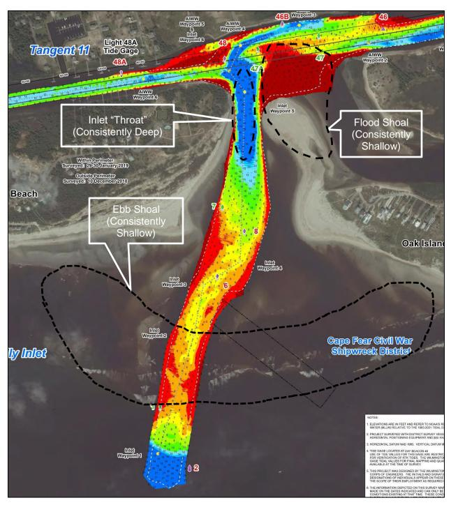
Figure 1-4. Inlet Throat, Flood Shoal and Ebb Shoal at LWF Inlet (Image Source: USACE Wilmington Navigation Branch)
