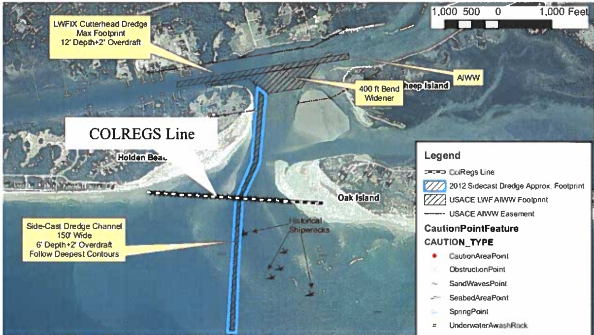
Figure 2-26a. LWF Inlet USACE Dredging Projects Include the Outer Channel (sidecaster dredged) and the LWFIK (cutterhead dredged)
