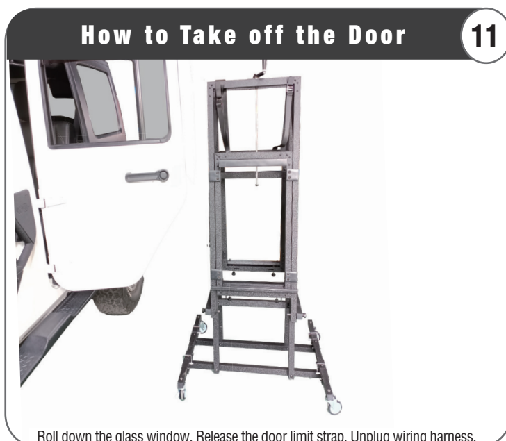
Roll down the glass window. Release the door limit strap. Unplug wiring harness.
