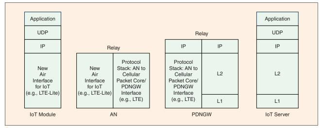
**FIGURE 4** The protocol stack for IoT air interface.
