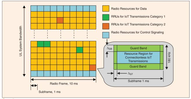
FIGURE 5 The radio resource grants for IoT transmissions in a 10-MHz LTE UL band.
