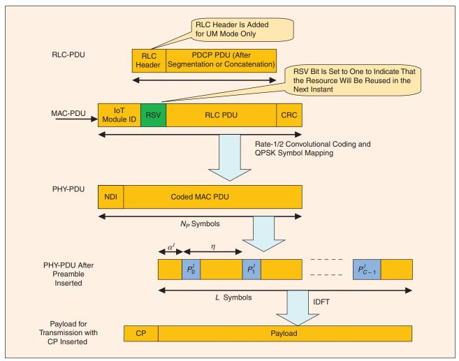
FIGURE 7 The PUSSCH payload transmission format.
