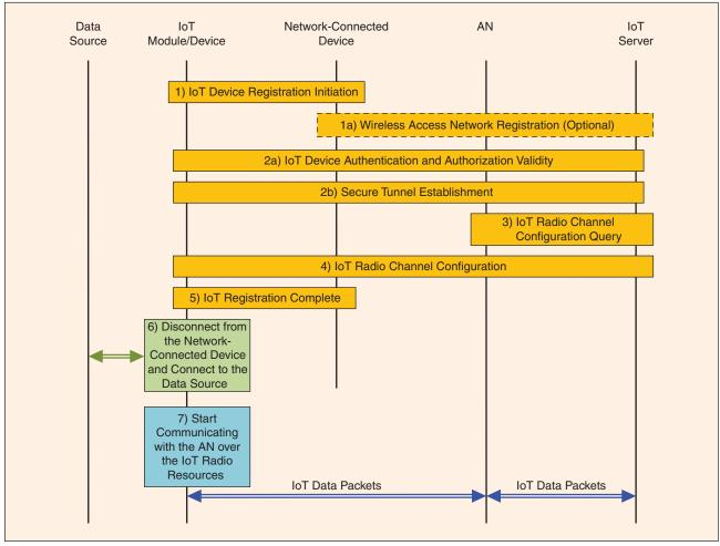
**FIGURE 3** The IoT module setup procedure.
