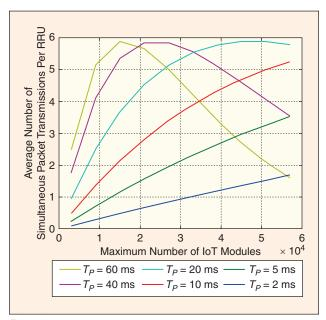
**FIGURE 9** The performance of the simultaneous access contention mechanism.
