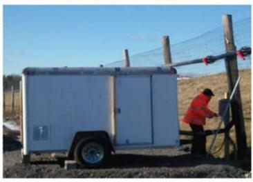
Connet unit to Power: 460/3/60, 20.5 Amps Service 4 wire 10 Gauge SO
