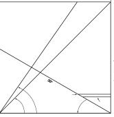
A plexi with 45°, 55°, 30° lines and a marker for 3cm and 3.5 cm drawn on or etched in. You will find a template in this folder under "Angle Guide Template"
