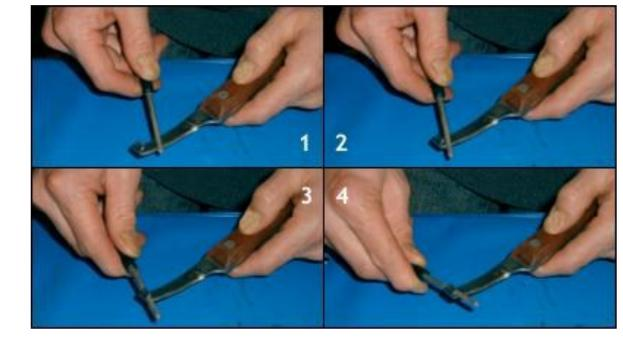
The direction of the stroke is both along the blade and across the edge. The handle of the sharpener is closer to the blade at the end of the stroke than at the beginning and it starts above the plane of the blade but, because I'm following the contour of the hook and keeping it at the same angle all the way around the hook, it ends below the plane of the blade.
