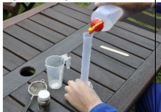
Accurately measure the amount of flotation solution required for the test.
