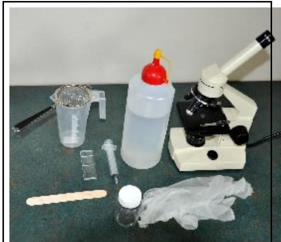
The minimum equipment needed to conduct an egg count. An extra measuring beaker and a small set of scales capable of accurately measuring 4 grams would be an advantage.
