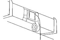
6. Unit may be taped with aluminum HVAC tape to provide complete seal.
