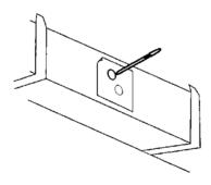
2. Using the appropriate template included, mark location for installation. (DW8000 is shown)
