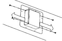
7. Replace cover and secure with the original four (4) screws.
