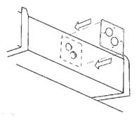
4. Place the mounting plate squarely into place and fasten to duct work with metal screws.
