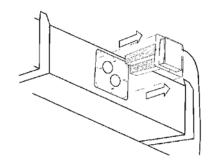
3. Remove the two bolts on either side of the cell to remove the cell from the ballast assembly.
