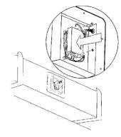
5. Place new ballast into original location and fasten the two (2) locking nuts into place.
