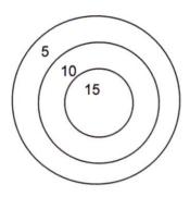
5# Salt / ft<sup>3</sup> = 20,000 grain removal / ft<sup>3</sup> resin 10# Salt / ft<sup>3</sup> = 25,000 grain removal / ft<sup>3</sup> resin 15# Salt / ft<sup>3</sup> = 30,000 grain removal / ft<sup>3</sup> resin
