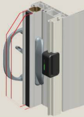
A-1 Vertical mullion for multi-panel units. Aluminum reinforced and secured with stainless steel screws through metal plate and directly into reinforcement.
