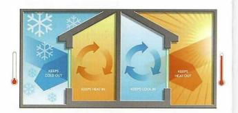
Low-emissivity (low-E) glass helps control the transfer of heat to help make buildings more comfortable, energy efficient and filled with natural light.
