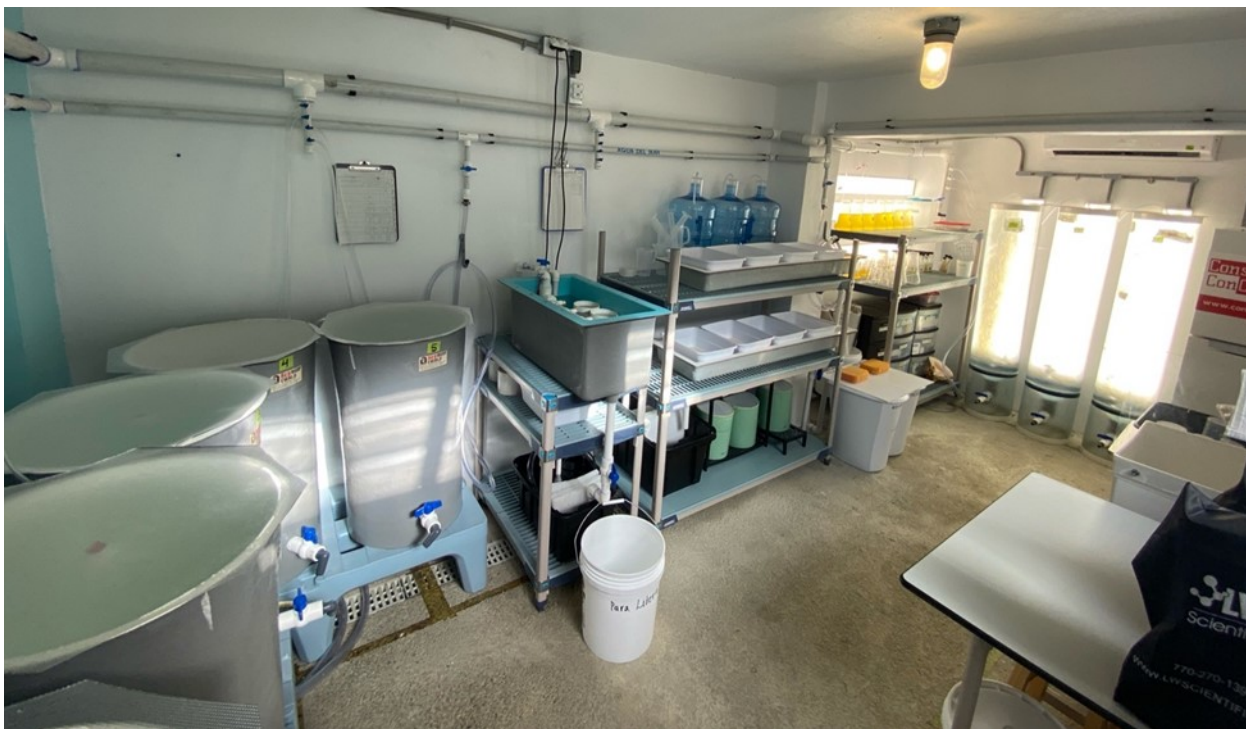
Figure 1. The Puerto Rico Queen Conch Hatchery located at the Naguabo Fishing Association. Hatchery includes egg incubator, larval tanks, metamorphosis system, microalgae culture, sink, and microscope table. Systems include filtered and UV-sterilization seawater, aeration, and freshwater.
