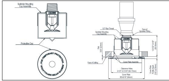
Properly installed sprinklers must have a nominal 3/32" (2.4mm) air gap between the lip of Cover Plate and the ceiling. The air gap is necessary for the proper operation of the sprinkler. If the ceiling is to be painted after installation of the Cover Plate Assembly, care must be taken to ensure that new paint does NOT seal off the nominal 3/32" (2.4mm) air gap.
