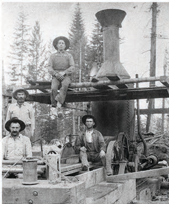
Steam donkeys are steam engines that turn a large winch, or capstan. During the late 1800s and early 1900s they were used in timber harvesting to pull logs out of the forest. c. 1890 at Pine Ridge.
