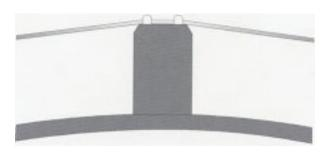
slight upward curve which is called crown. The downbearing and crown must be very precise. It takes very little change to dramatically compromise the tone.
