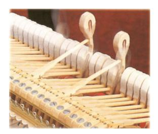
Just as doors and drawers become loose in dry air, the keys of your piano may rattle or become mechanically noisy. When the wooden action parts shrink from dryness, they become loose and can move around. This will lead to premature wear of these parts and costly repairs in the future.
