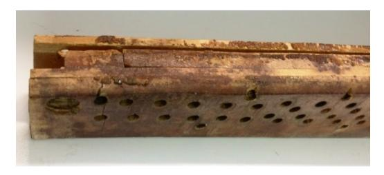
The up and down cycling of humidity can also cause the layers in the pinblock to delaminate. This is virtually always accompanied by cracks developing within the layers themselves. The cost of this type of repair can often exceed the value of the piano.
