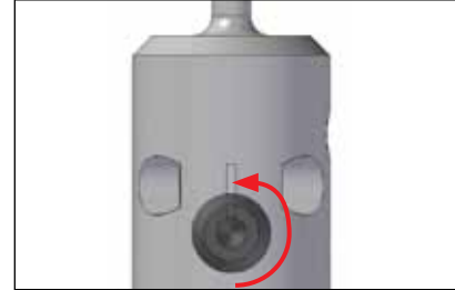
Turn back the excenter by 180° until the groove of the excenter is aligned with the groove in the tool body.
