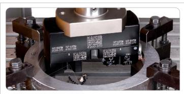
UP TO ,600 SFM This system is made of lightweight aluminum and can be used for both rough and fine boring, as well as OD turning and grooving applications. It can operate at high speeds of up to 6,600 SFM, and is designed to be completely safe with pinned-to-fit mounting. Additionally, the system comes equipped with coolant supply through all components direct to the cutting edge.
