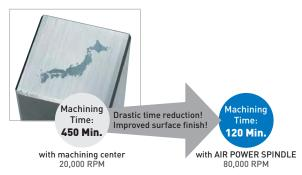
Map of Japan milled with R .004" ball nose end mill. Material: Prehardened Steel HRC40
