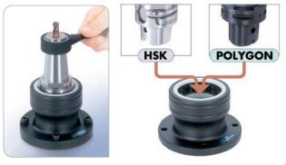
Ideal fixture for the set-up of cylindrical shank tool holders.
