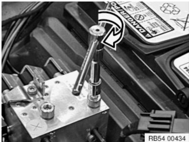
Fig. 94: Opening Screw On Hydraulic Unit Courtesy of BMW OF NORTH AMERICA, INC.
