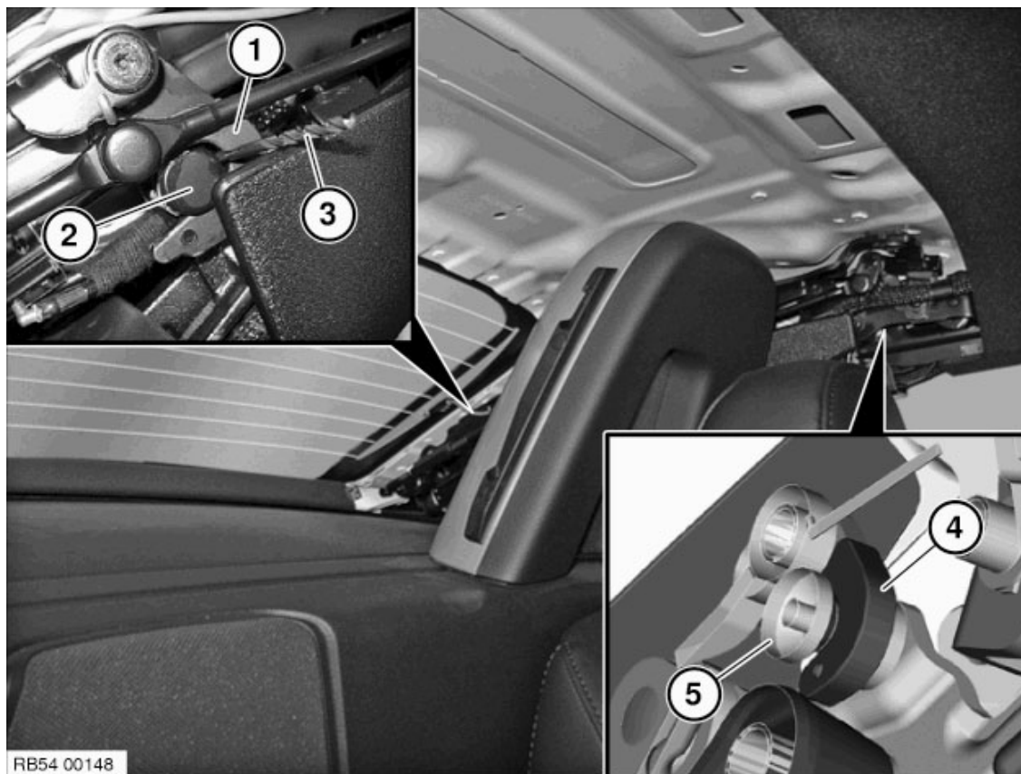
Fig. 27: Checking Gap Dimensions Courtesy of BMW OF NORTH AMERICA, INC.
