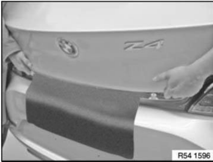
Fig. 176: Positioning Helper On Both Sides Of Rear Module Courtesy of BMW OF NORTH AMERICA, INC.
