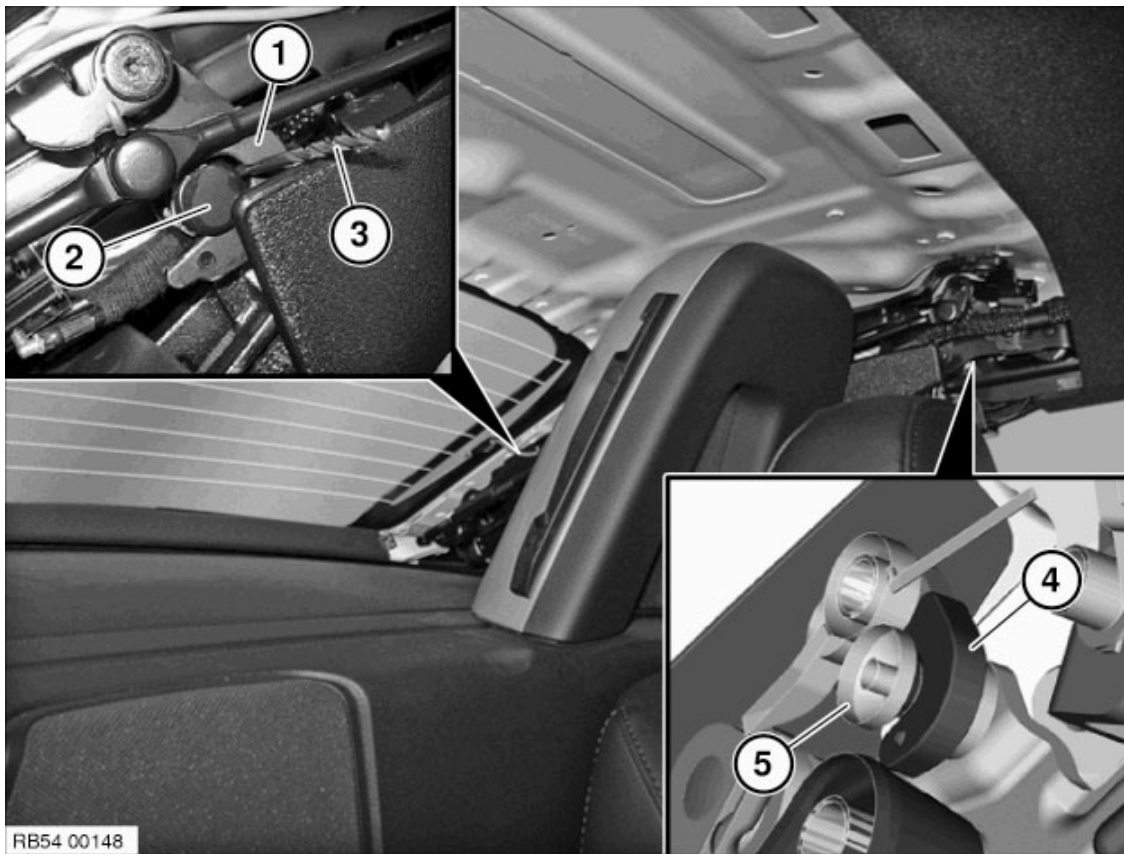
Fig. 27: Checking Gap Dimensions Courtesy of BMW OF NORTH AMERICA, INC.
