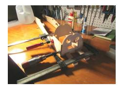
Engine carriage glued between fuse sides
