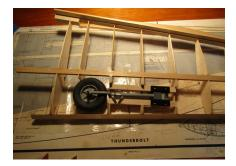
Retract test-fitted into mounting beams
