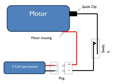
Wire connection to the motor housing on left and I used a screw to hold the terminal lug to the spade clip on the motor.
