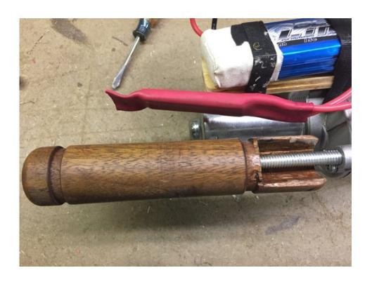
Here is the handle slipped over the threaded rod. Nut both ends to hold it in place.
