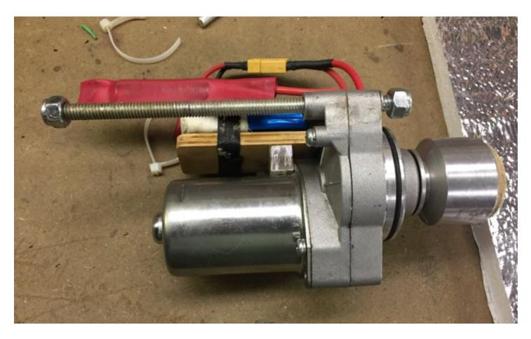
Here is the wooden handle I made showing the cutout so it fits over the housing. The cutout on the right allows the wood to fit over the starter. This is optional; I did it to make it look nicer. The two grooves were added to capture the zip tie that holds the switch to the handle
