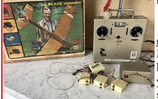
Finally in 1972, after lots of saving I got my first radio—a World Engines Blue Max MKII 6 channel radio set which I still have today. This was like a Heath Kit and you actually had to assemble it including soldering all the components and wiring.
