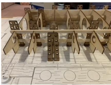
Magnets at the base of each rib guide grips to the metal sheet beneath the plans. Ribs are held in perfect 90° alignment for gluing.
