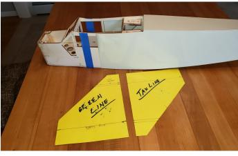
Since I was changing colors along the length of the fuse, I measured and cut stencils (see picture) that allowed me to neatly overlap the material in a uniform manner. When applying UltraCote over UltraCote, eliminating bubbles is essential. I first moisten the base
