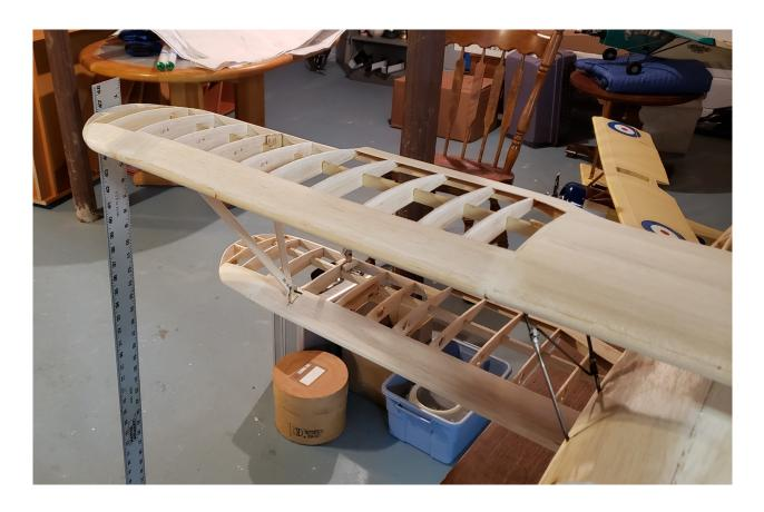
The plans call for simply screwing the top wing onto the cabanes. I am not sure how one would make all the adjustments when you do that, so I instead chose to solder lugs onto the cabanes and use 6-32 bolts attached to blind nuts embedded in the wing.
