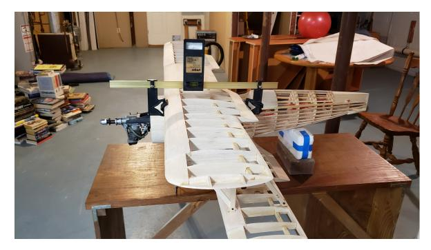
When both wings were attached and rechecked for correct measurements, I fabricated the outer struts from basswood, 4-40 bolts, and blind nuts. Now it's time to begin the covering process.
