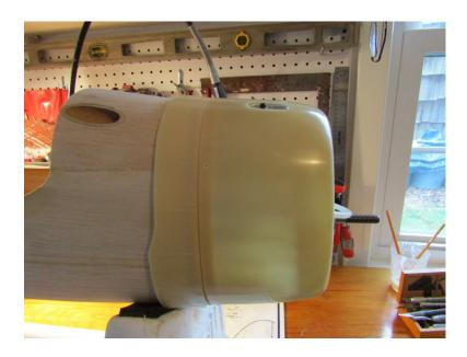
In order to create the needed exit-hole, I began with a piece of thin, transparent plastic sheet. I cut out a hole whose diameter was the same diameter as the elbow. Then, the elbow was placed through the hole of the sheet and reattached to engine. Tape was provided to mount the sheet onto the fuselage. The position of the elbow was carefully considered with the muffler attached before the tape was firmly pressed into place.
