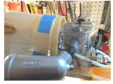
Keeping the plastic sheet secure and unmoved on the fuselage, the elbow is carefully removed and the cowl is then replaced.
