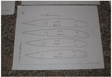
Using a little math, I determined that 1/2 scale is really 1/2 scale times 0.8333. I had access to a nice office-size printer so I asked it to reduce each sheet by that amount. I cut a few printed pieces that matched my plans and laid them over to check the sizing. I tried six
