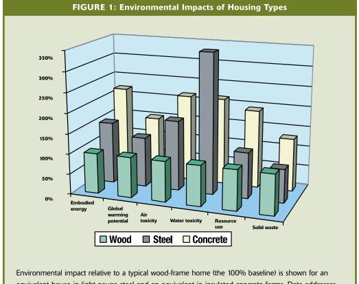
Environmental impact relative to a typical wood-frame home (the 100% baseline) is shown for an equivalent house in light-gauge steel and an equivalent in insulated concrete forms. Data addresses the life-cycle portion from resource extraction through construction and does not include environmental impacts of building occupancy and demolition.
