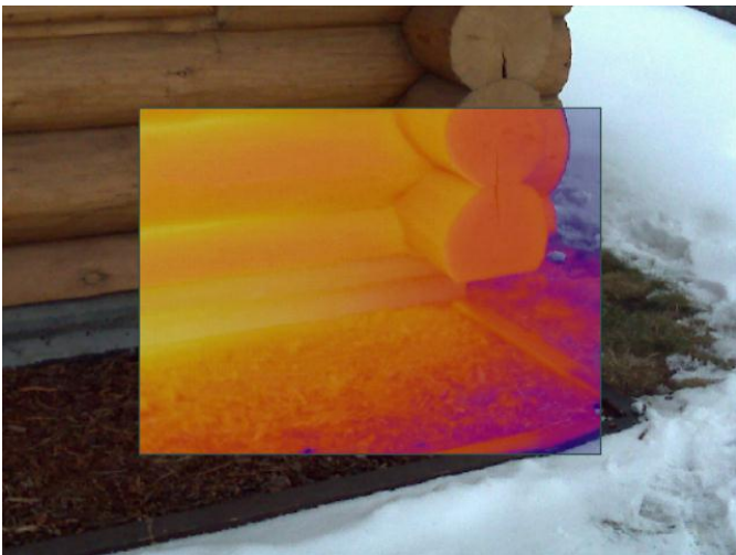
Fig.3.12 IR photo of the foundation (crawl space) wall and log wall interface during depressurization (left) and pressurization (right), showing air leakage through the crawl space vent during pressurization.
