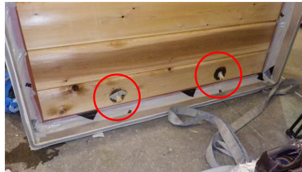
Fig.2.4 Log home test wall with plug in the vent holes sealed.
