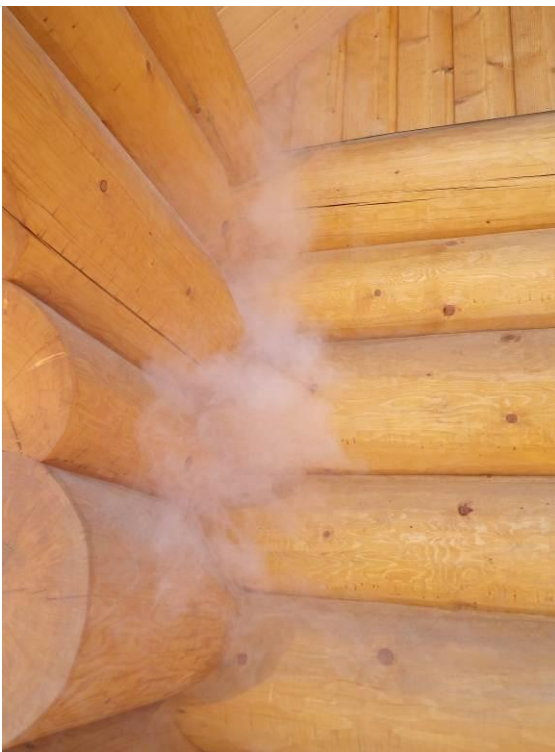
Fig.3.28 Smoke leakage observed at log wall corner joint during pressurization.
