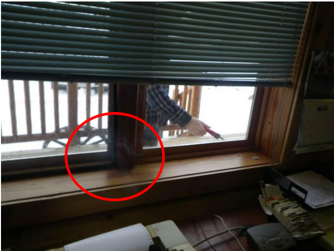
Fig.3.4 Smoke infiltration observed at operable windows during smoke pencil testing from the exterior under depressurization.
