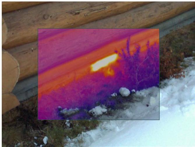
Fig.3.12 IR photo of the foundation (crawl space) wall and log wall interface during depressurization (left) and pressurization (right), showing air leakage through the crawl space vent during pressurization.
