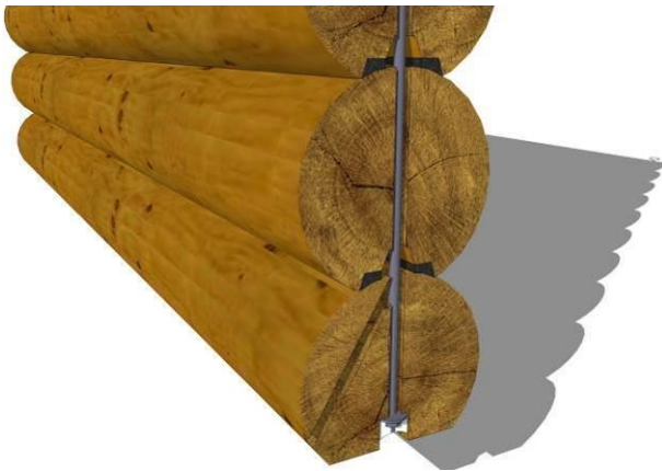
Fig.2.3 Rendering of how the lateral groove and venting of the log home test wall was achieved.
