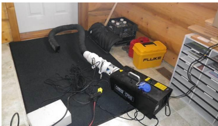
Fig.3.2 Theatrical fog machine smoke testing apparatus.
