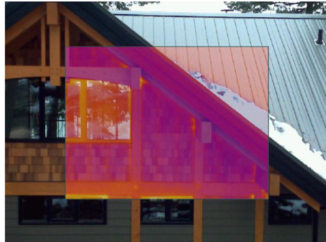
Fig.3.21 IR photo of the gable and roof overhang during depressurization (left) and pressurization (right), showing air leakage at joints during pressurization.
