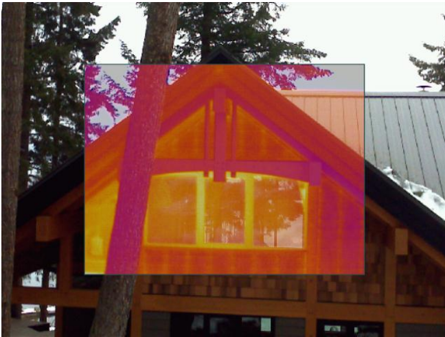
Fig.3.21 IR photo of the gable and roof overhang during depressurization (left) and pressurization (right), showing air leakage at joints during pressurization.
