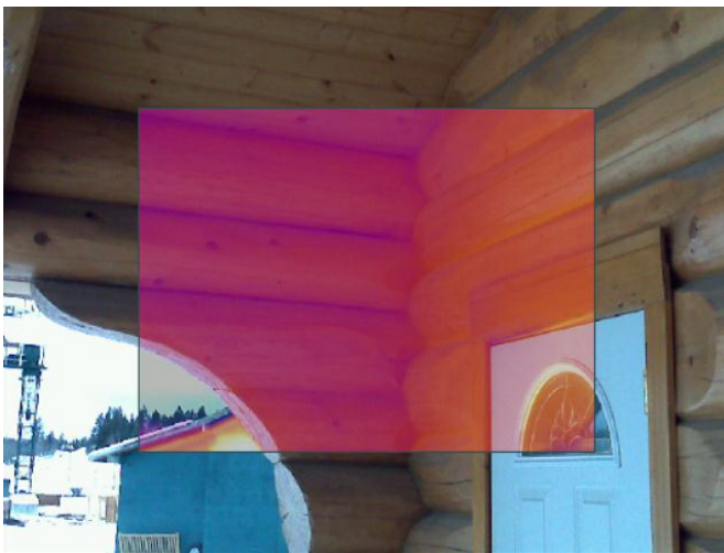
Fig.3.7 IR photo of a joint during depressurization (left) and pressurization (right), showing air leakage through the joint during pressurization.
