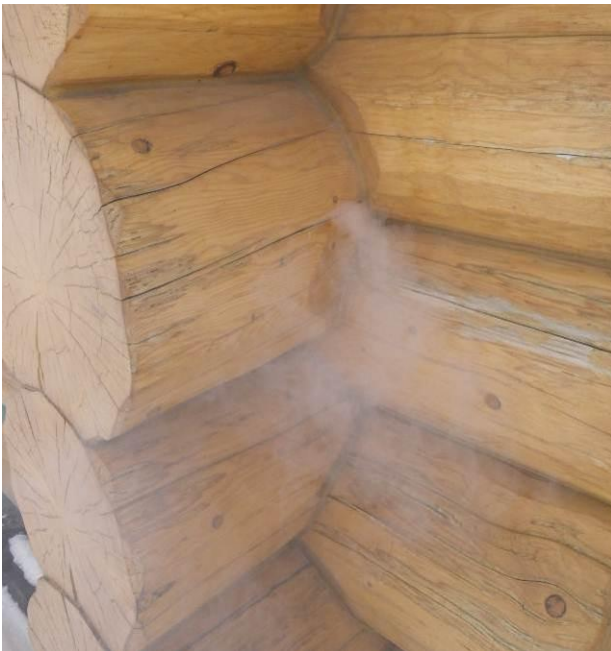
Fig.3.5 Smoke infiltration observed at corner joints and exterior door during smoke testing from the interior under pressurization.
