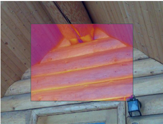
Fig.3.11 IR photo of the gable and roof overhang during depressurization (left) and pressurization (right), showing air leakage at the joint during pressurization.
