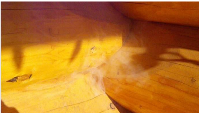
Fig.3.30 Smoke leakage observed at log wall corner joint (left) and at window jamb (right) during pressurization.
