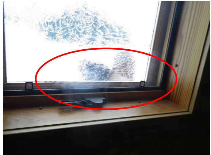
Fig.3.4 Smoke infiltration observed at operable windows during smoke pencil testing from the exterior under depressurization.
