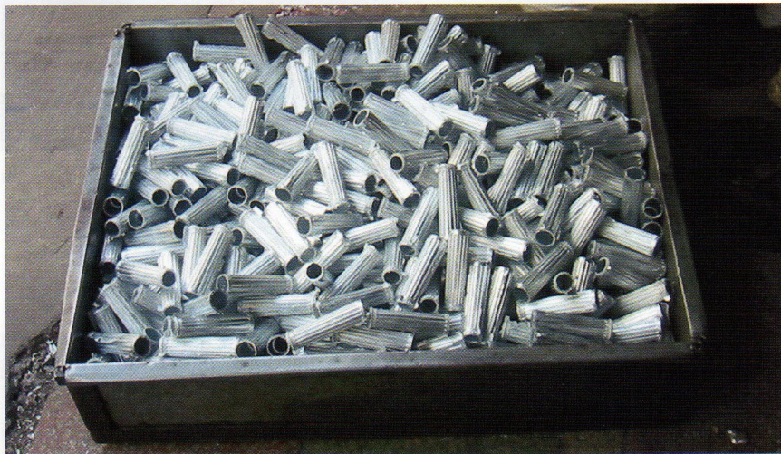
The case of the Social Light is first molded and then plated before the exterior case is applied.
