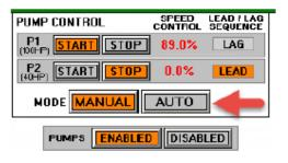
2) Both High Service Pumps are available and programmed with SCADA to adjust VFD speed to meet target pressure set points. The Sr. Chief Operator, Alan Allen, and Dave Nista will be able to change the target pressure set points and the response time between changes.
