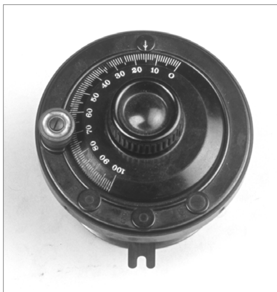
Figure 5-9. Tuning condenser, third version (terminal bosses still present).
