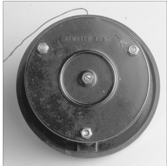
Figure 5-13. Tuning condenser, sixth version, showing Bakelite rear plate with "ATWATER KENT" molded into the plastic.
