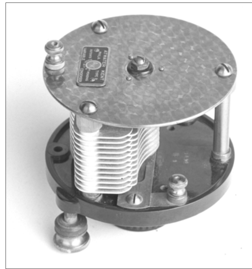
Figure 5-4. Type P tuning capacitor #4165, side view showing ID plate and terminals.
