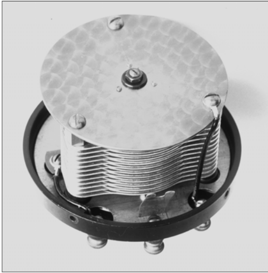
Figure 5-2. Rear view of Type E tuning condenser, showing jeweling pattern and ground clip.
