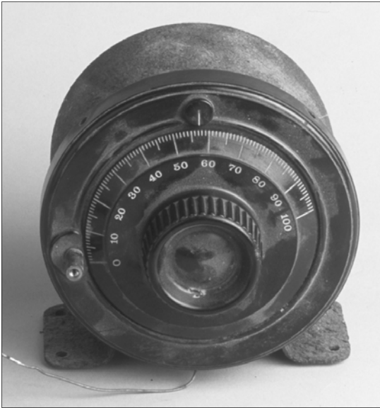
Figure 5-11. Tuning condenser, sixth version.
