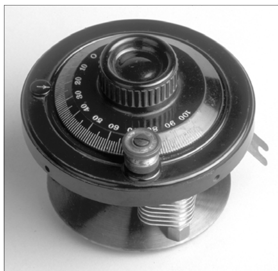
Figure 5-10. Tuning condenser, fourth version.
