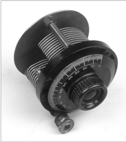
Figure 5-5. Type P tuning condenser, front view, showing rotor terminal and proper dial orientation.
