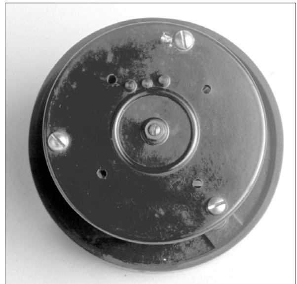
Figure 5-14. Tuning condenser, sixth version, without the Atwater Kent name on the Bakelite rear plate.
