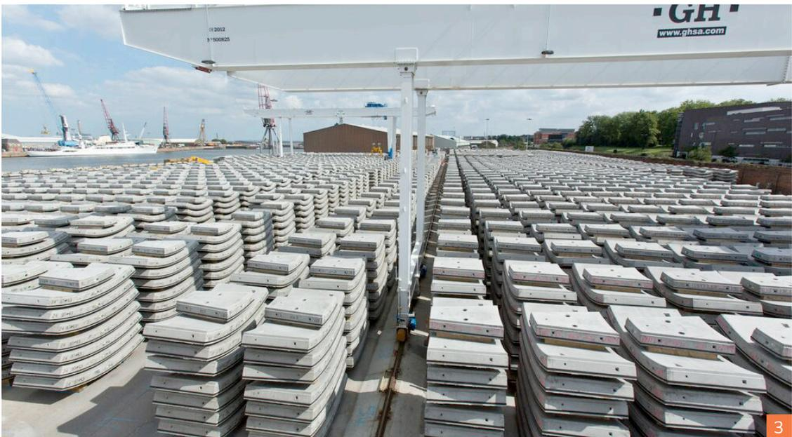
Kent Wire's Products: 1. Steel reinforcements. 2. Anthony Gormley RA show. 3. Tunnel lining sections for Cross Rail.
