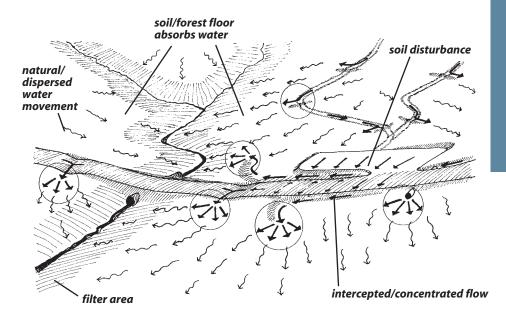
One way BMPs minimize impacts to water quality is by dispersing concentrated water flow. Circles indicate where BMPs disperse flow to the undisturbed forest floor.
