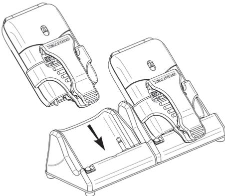
**Note:** The NBC 9-3-2 Digital Fast Charger will maintain batteries in a fully charged state, and the M-216 and PR-216 can be stored in charging bays indefinitely while the steady green LED is on. Periodically open the battery compartment on stored COMTEK units to check for battery leakage. If a Ni-MH battery is leaking, it must be discarded.
