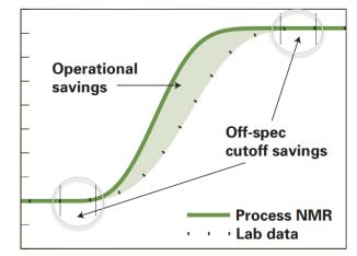
Fig 1. Operational transitions showing continual process measurement versus hourly laboratory results
