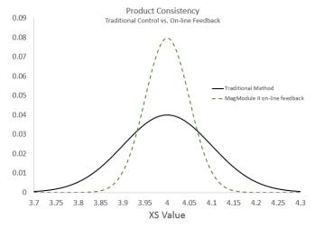
Fig 2. Product consistency variation control based on MagModule II online feedback
