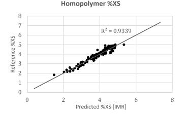
Fig 3. Magneflow® technology compared with lab reference data for the %XS content in
