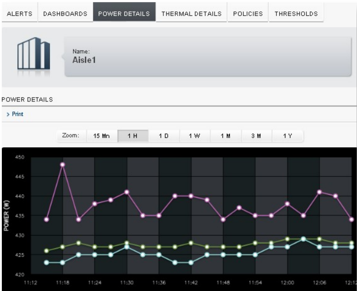
Figure 10 OpenManage Power Center power monitoring GUI
