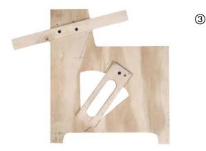
To the left is an Atwood-Hamlin Bracket Jig with upper sticks and bracket angle that will need to be adjusted. Once these are adjusted, by following the instructions below, you will be able to use the jig as a template for each pew keeping the installation process consistent.<sup>®</sup>
