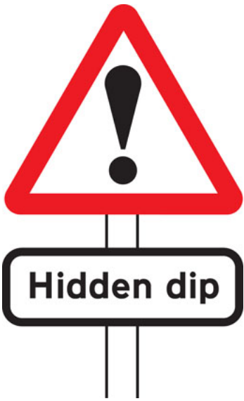
Other danger; plate indicates nature of danger
