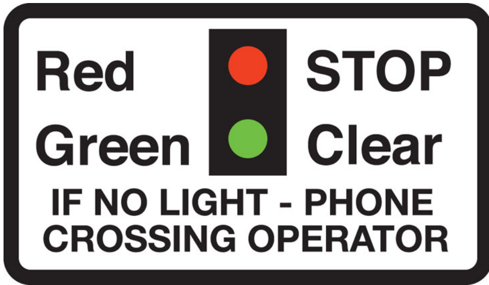
Miniature warning lights at level crossings
