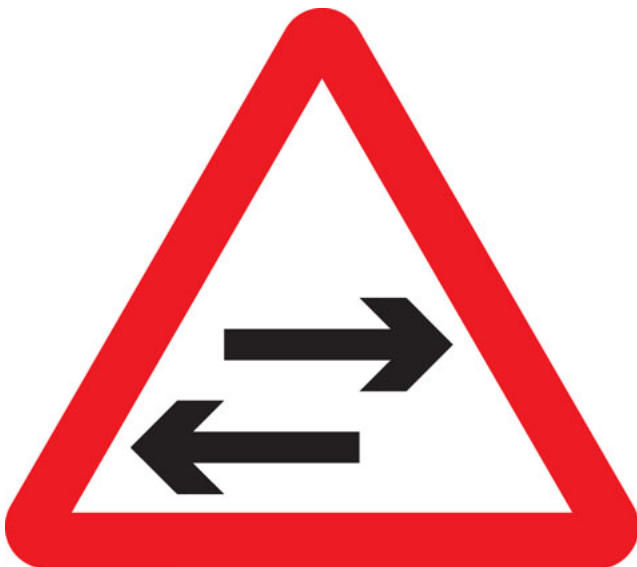
Two-way traffic crosses one-way road
