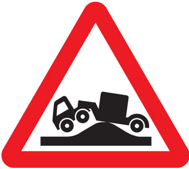
Risk of grounding
