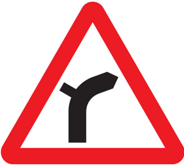
Junction on bend ahead
