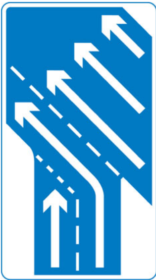
Traffic in right hand lane of slip road joining the main carriageway has priority over left hand lane
