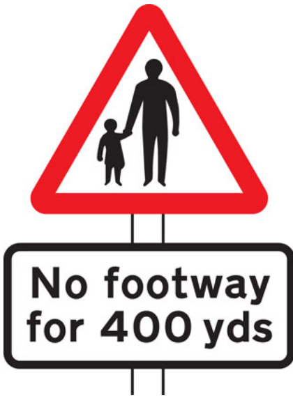
Pedestrians in road ahead
