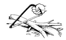
*Bow Saw* - Not strictly an axe of course, but often used in conjunction with axes for preparing firewood. You may come across a variation of the bow saw, for example, the bush or 'sandvic' saw. Bow saws are used for wood too large for using a hand-axe and are often safer and easier than the felling axe for cutting small timber. They should be greased to prevent them from rusting and, as blades are relatively cheap, it is advisable to replace the blades rather than attempting to sharpen them!
